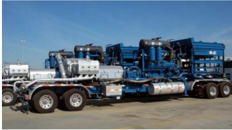
Truck with positive displacement pump.
