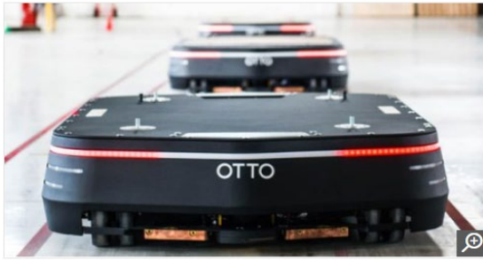
OTTO 1500 self-driving vehicles for materials transport.
