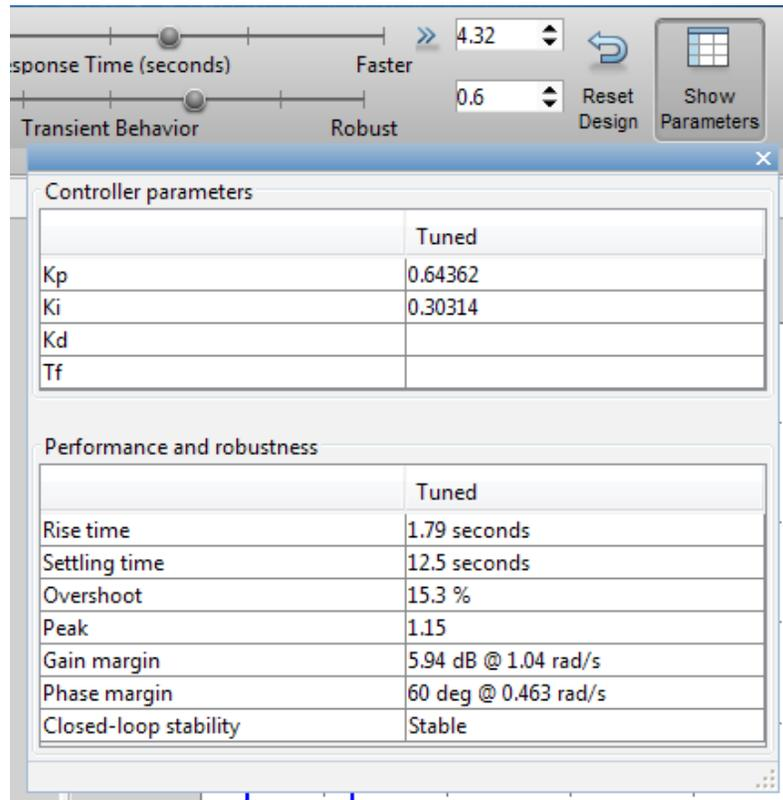
Because we increased the bandwidth, the step reference tracking response becomes more oscillatory. Additionally the overshoot exceeds 15 percent, which is usually unacceptable. This type of performance tradeoff between reference tracking and disturbance rejection often exists because a single PID controller is not able to satisfy both design goals at the same time.
