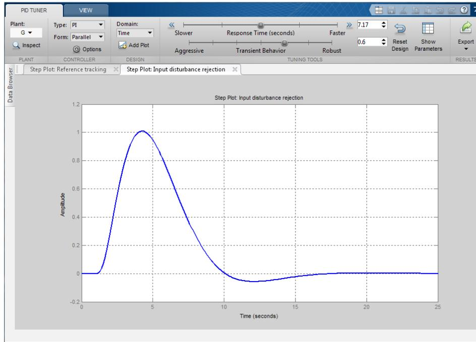
Tile the plots to show both the reference tracking and input disturbance responses. Move the response time slider to the right to increase the response speed (open loop bandwidth). The  $K_i$  gain in the **Controller parameters** table first increases and then decreases, with the maximum value occurring at 0.3. When  $K_i$  is 0.3, the peak deviation is reduced to 0.9 (about 10% improvement) and it settles to less than 0.1 in about 6.7 seconds (about 25% improvement).
