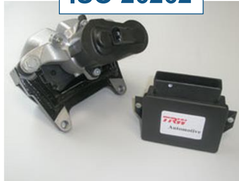
TRW Germany Electronic parking brake control system
