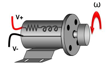
$$V_{in} = K_b \omega + i_m R_m + L_m \frac{di_m}{dt}$$
