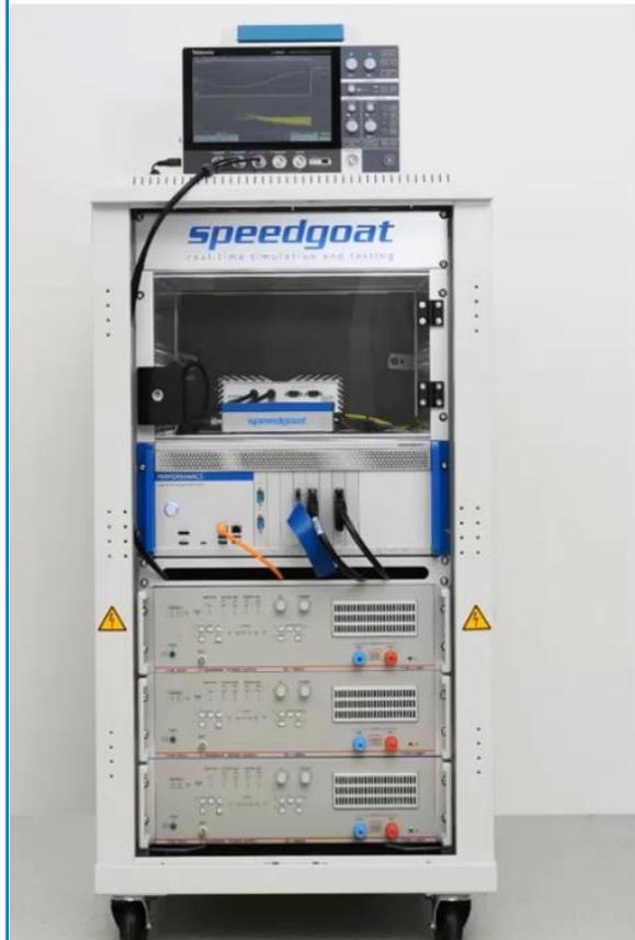
Speedgoat Power HIL Testbed
