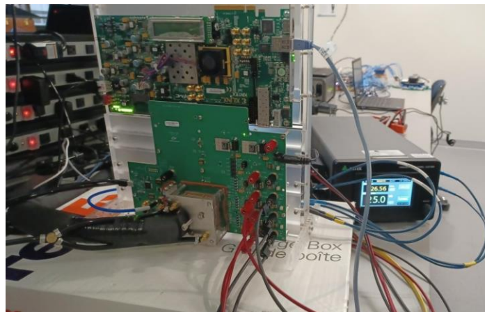
Fig. 15. BER lab measurement setup
