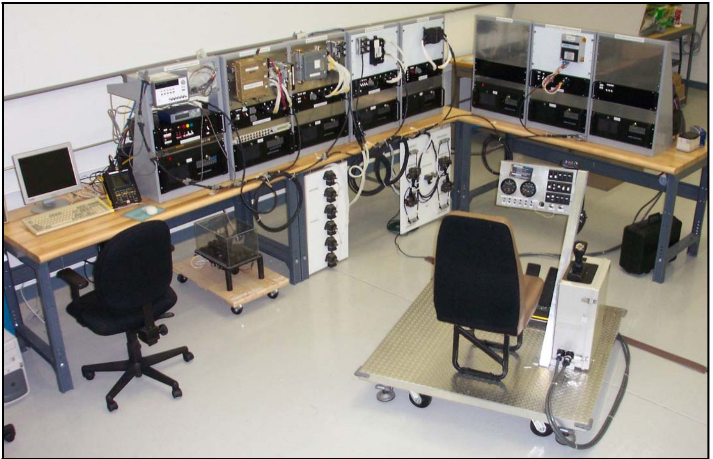
Exhibit 1 – HIL Simulator Test Bed
